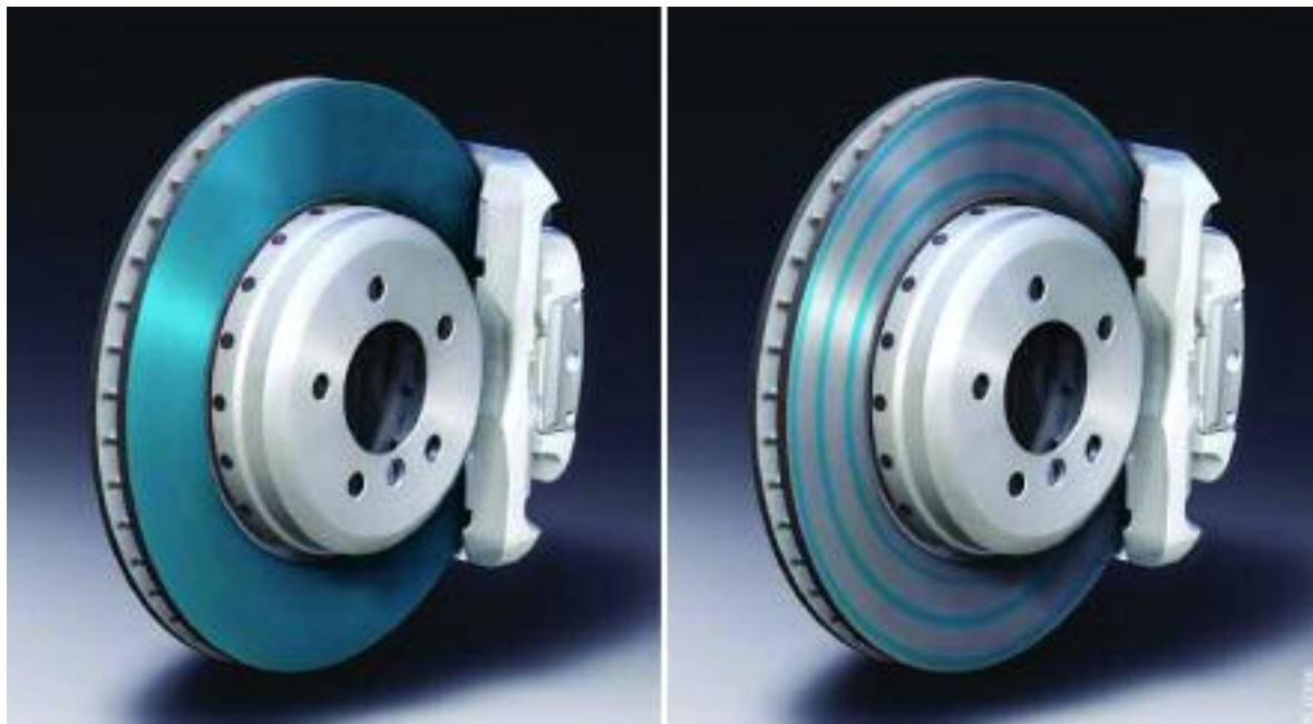
Left disc with water film before dry braking Right brake disc after dry braking
